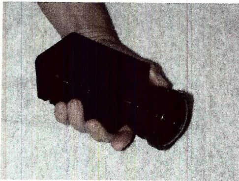
Figure 10: One of two airborne fisheye systems designed for use with a UAV. The first figure illustrates the camera that acquires images near 1.6 \mu\text{m} in the NIR, and the second image illustrates data from the visible system near 650 nm.
